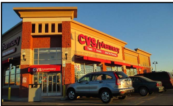
Pedestrian scale – awnings, elevation relief, textures, shadow, color, display, sconces, brick
