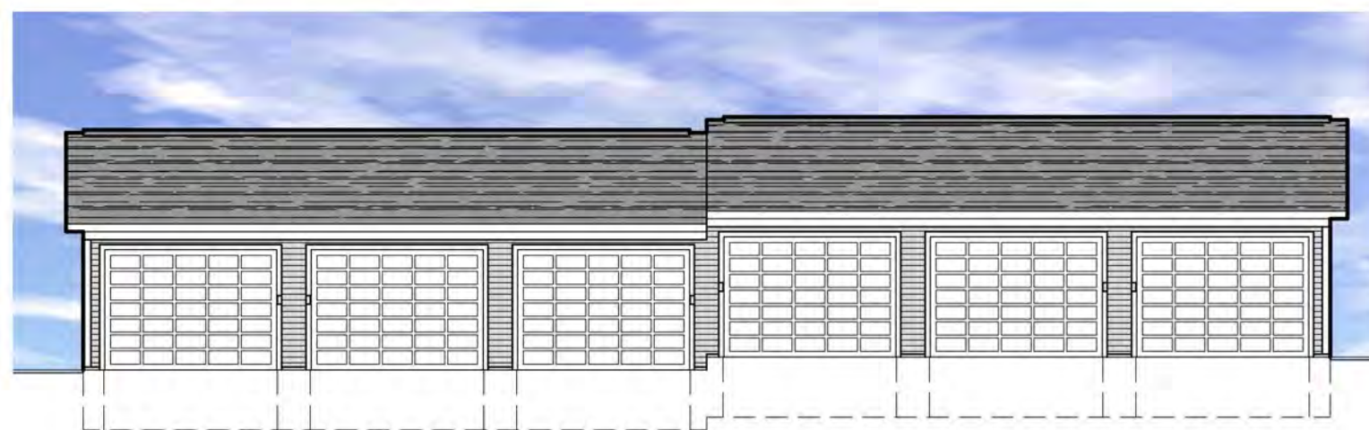
6-Stall Front Elevation w/ 2 Finish Floor Elevations
