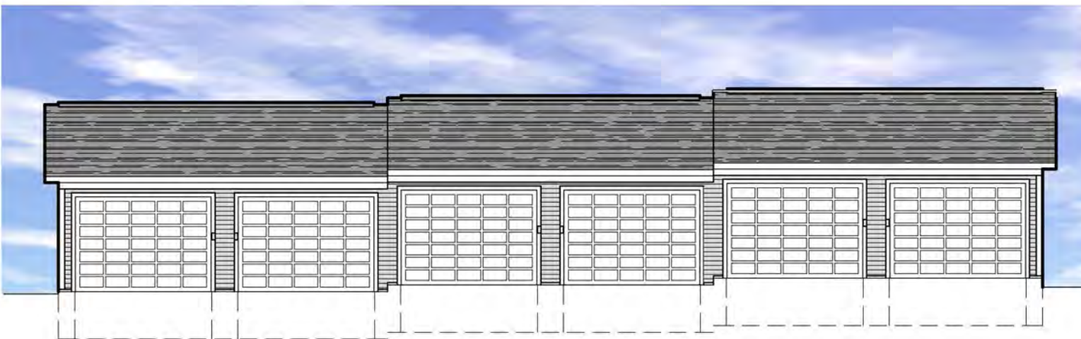
6-Stall Front Elevation w/ 3 Finish Floor Elevations
